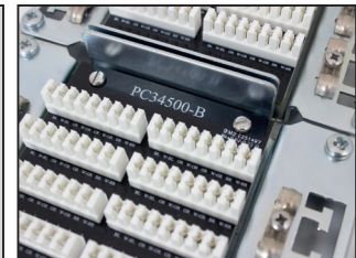
ZTB Internal view showing PCB trays with cable anchor points and shielding clamps
