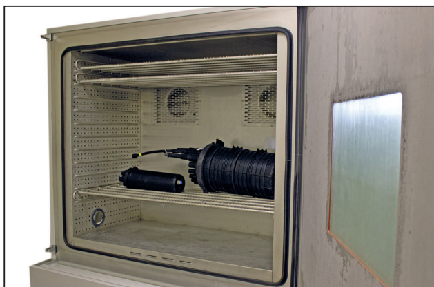
Image 6: Environmental Chamber shown with door open
