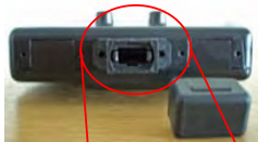
3.2. MTP adaptor on rear of cassette with dust cap removed
