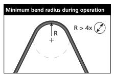
Bend Radius during operation shall never be less than 4 times the diameter of the cable.
