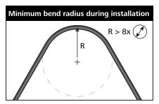
Bend radius during installation shall never be less than 8 times the diameter of the cable.
