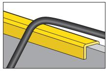
Guides/runners/edge protectors shall be used on all corners to protect cables and maintain minimum bend radius.
