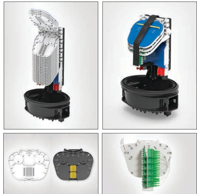
Top Left: CFN 27 port M-length shown with SC-B trays. Top Right: Connectorised CFN 27 port S-length shown with 2 x SE-IR trays and 1 x connectorised tray with LC/APC QD adaptors. Bottom Left: Variety of trays available including SC-B and SE. Bottom Right: Rear view of connectorised tray with LC/APC connection.
