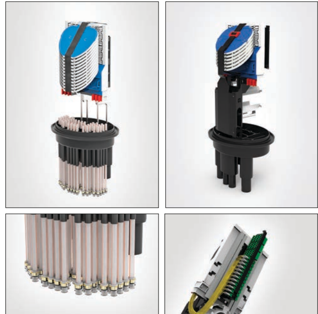
Top Left: FDN-IR 59 Port AB Length closure shown with 12 x SE-IR MKII splice trays and basket pre-tubed with microduct. Top Right: FDN-IR 59 Port AB Length closure shown with 24 LC APC connections.
