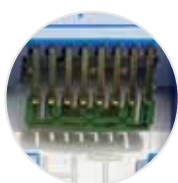
Contact set mounted PCB for optimised Cat 6A performance
