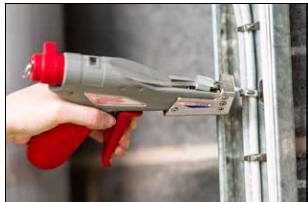
Hand tool designed to install stainless steel fasteners and fixings to the recommended tension
