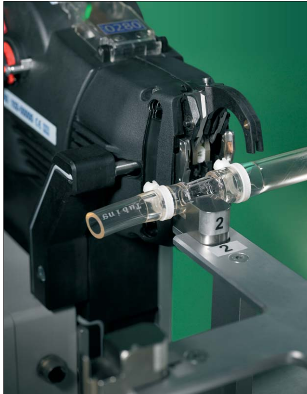
Exact positioning of cable ties.
